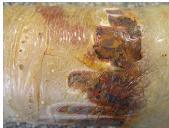
Figure L.2 — Corrosion protection reinstated between installed wrap and original paint coating; lack of corrosion protection leading to corrosion at edges of the repair
