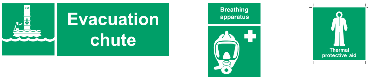
Figure 5 — Examples of combination signs using explanatory text panel supplementary signs (with and without internal borders)
