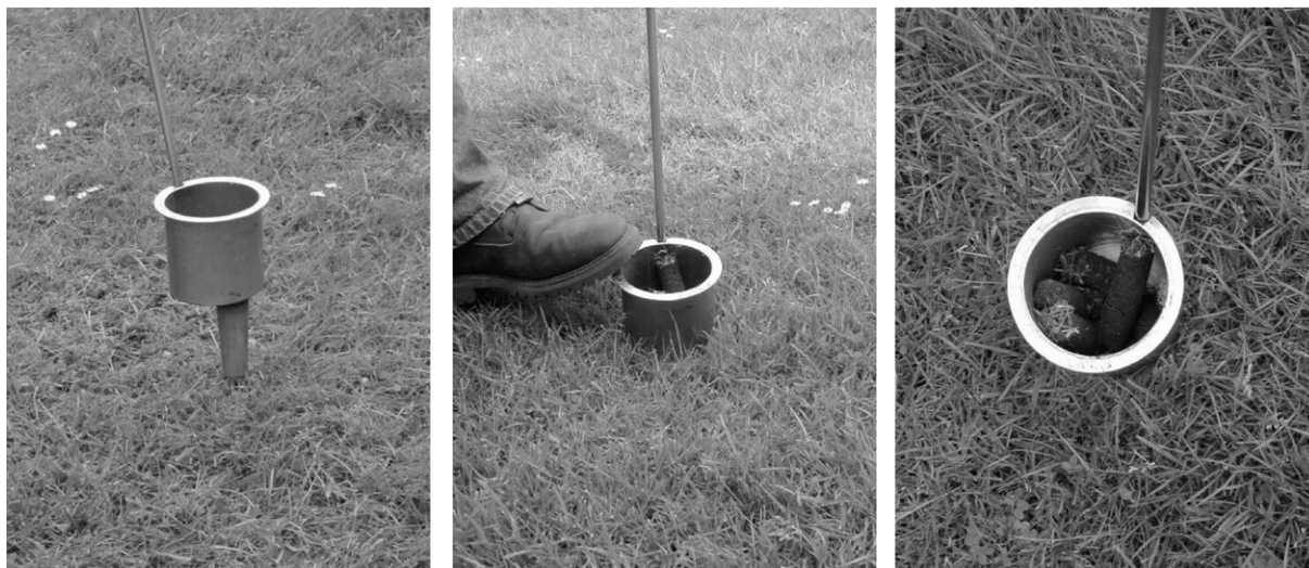
Figure A.1 — Grass plot corer in action
