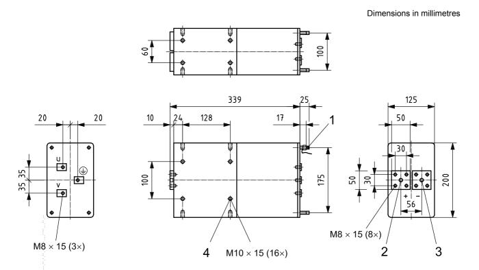
1 studs for connector box (4  $\times$  M8)
