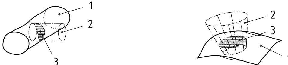
a) Cylindrical section volume, perpendicular to the axis of a cylinder b) Section volume limited by a ruled surface
