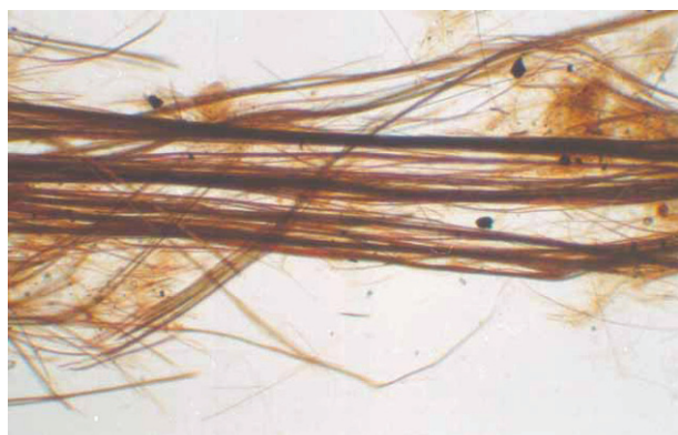
Figure D.17 — Heated crocidolite viewed in plane polarized light — Fibre length parallel to polarizer vibration direction
