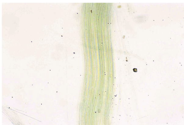
Figure D.44 — HSE actinolite in 1,640 RI liquid in plane polarized light — Fibres normal to polarizer vibration direction
