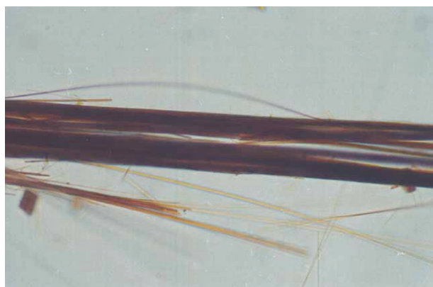
Figure D.9 — Heated amosite in 1,680 RI liquid viewed in plane polarized light — Fibre length parallel to polarizer vibration direction
