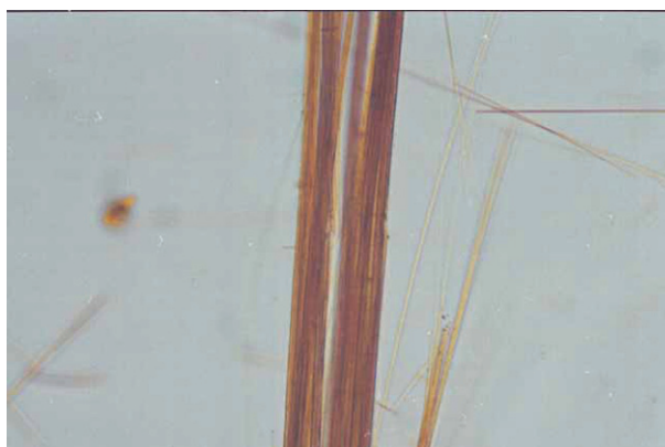
Figure D.10 — Heated amosite in 1,680 RI liquid viewed in plane polarized light — Fibre length parallel to polarizer vibration direction
