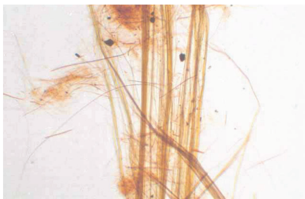
Figure D.18 — Heated crocidolite viewed in plane polarized light — Fibre length normal to polarizer vibration direction
