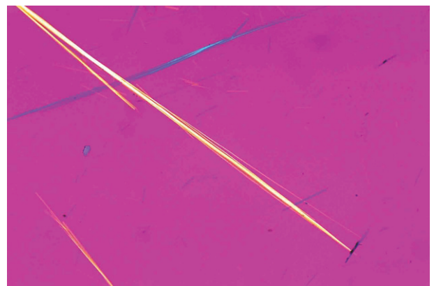
Figure D.28 — PLM micrograph of SRM 1867 actinolite in 1,630 RI liquid — Crossed polars with 530 nm retardation plate
