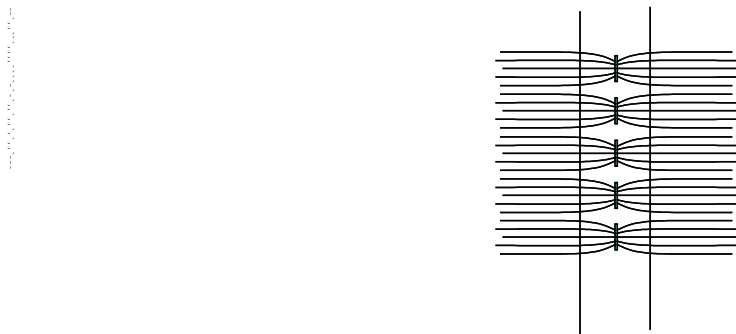
Figure A.4 — Induced thermal-constriction resistance caused by the construction of the heat source shown in Figure A.1
