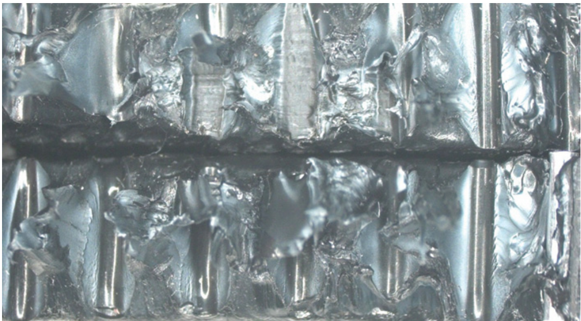
Figure 4 — Typical brittle fracture – side view
