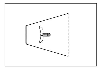
The front baffle has a hole to let the jet through. Recirculation is smoothed by the contraction generated by the oblique baffles; both on the return way and on the approach to the mixer. A perforated plate at the approaching flow entry reduces the large scale turbulence.
