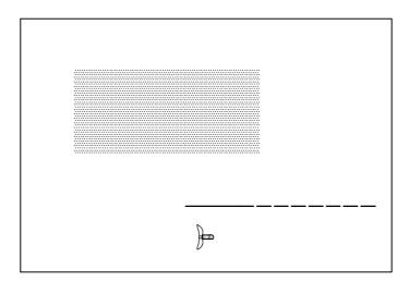
The large tank scale and some flow obstacles — schematically represented by dashes — reduce the momentum of the approaching return flow. A solid plate removes sideways return flow influence on the mixer. A perforated plate upstream of the solid plate reduces the sideways return flow influence on the approaching flow and partly deflects the return flow.
