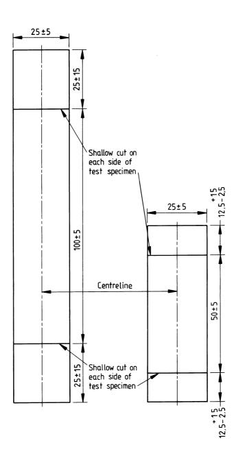
Figure 1 - Long and short test specimens for shrinkage, showing dimensions and positions of reference cuts
