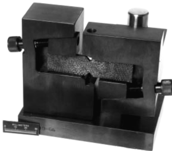
Figure 3 — Photograph of commercially available fixture for Iosipescu test
