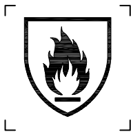
Figure 1 — Symbol ISO 7000-2417 to indicate clothing for protection against heat and flame
