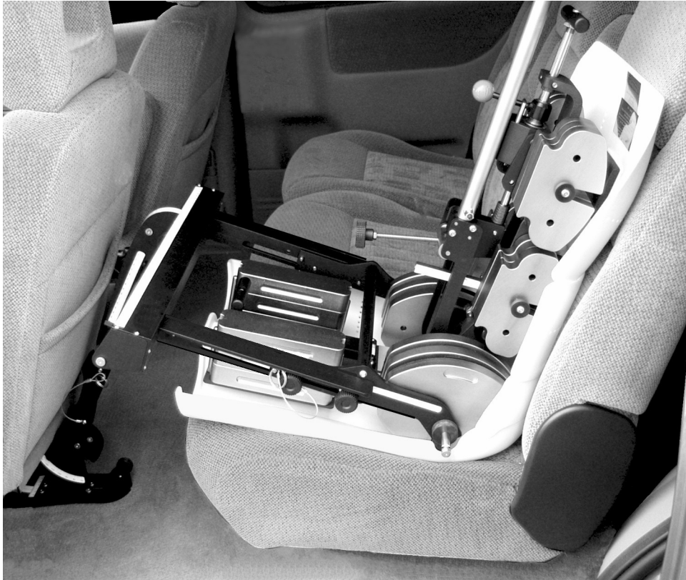
Figure 12 — H-point machine installed in rear outboard seat
