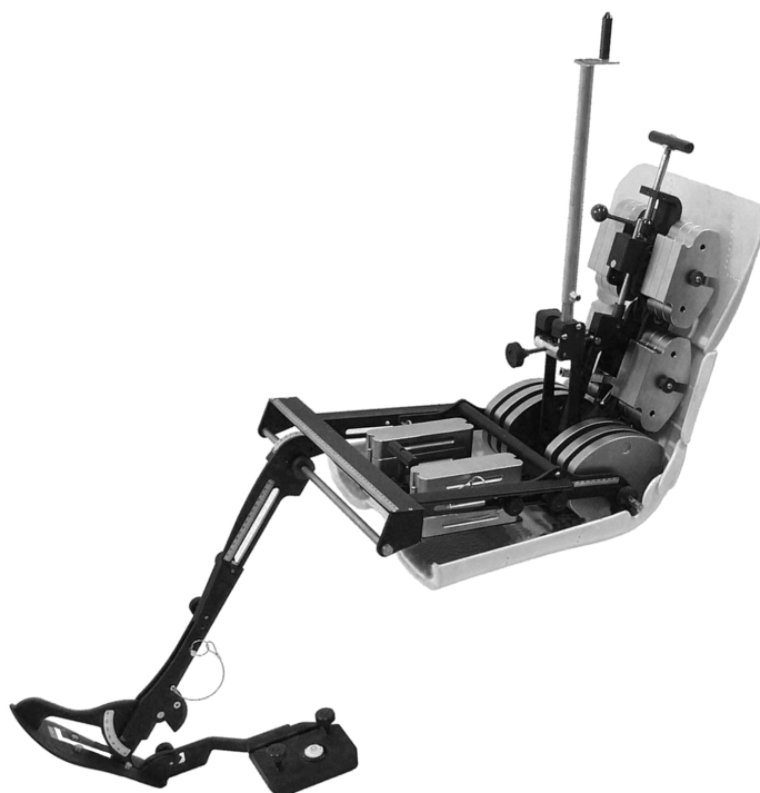
Figure 7 — Perspective view of HPM, including optional components
