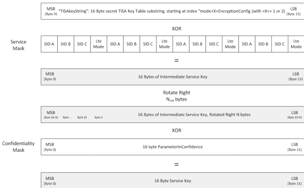
Figure 5 — Procedure for composing a Service Key, based on the secret TISA Key Table, transmitted service parameters and the ParameterInConfidence
