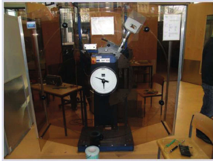
Figure A.2 — Testing equipment for ISO-V specimens — Instrumented pendulum — 300 J testing machine
