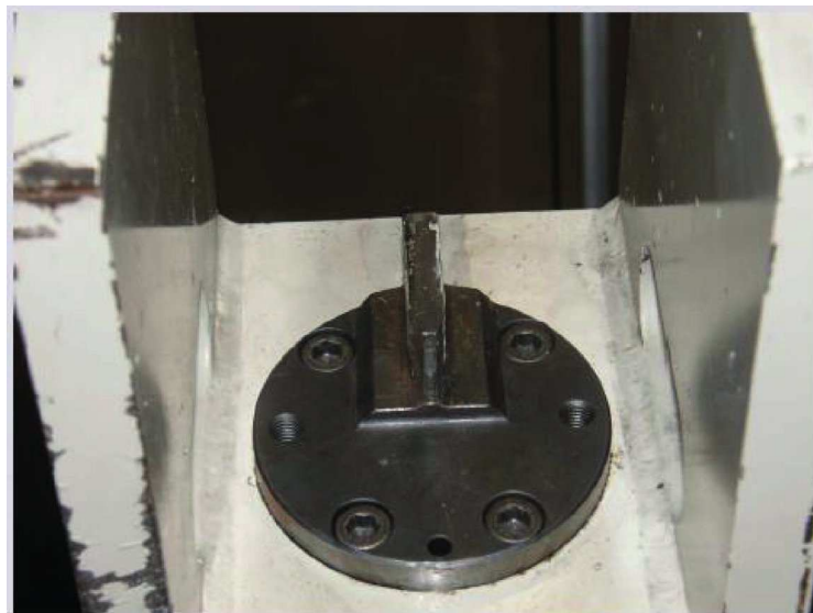
Figure A.3 — Testing equipment for ISO-V specimens — Instrumented peen
