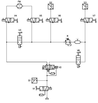
Key FM Flow meter S1 to S3 Pressure sensors Regulator under test R V Volume V1 Inlet shut-off valve V2 Cycling valve V3 & V8 Isolation valves V4 to V7 Sensor shut-off valves
