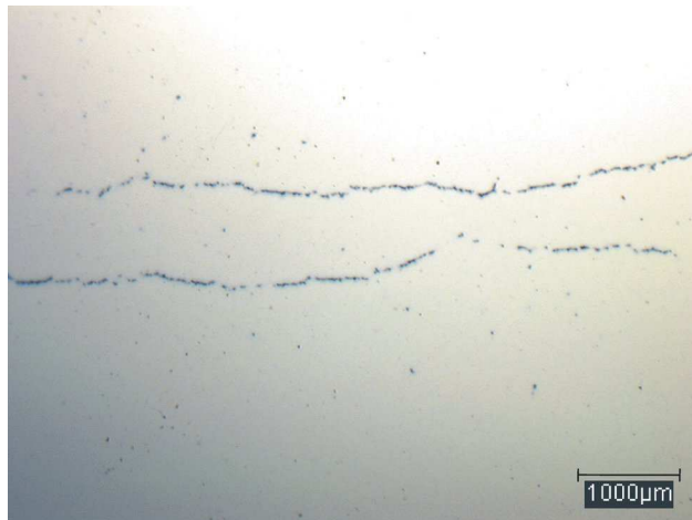
b) Hairlines, top view [corresponding cross section; see Figure 2 c) ]
