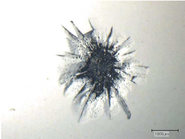
a) Pop-off resulting from impact on the rear side
