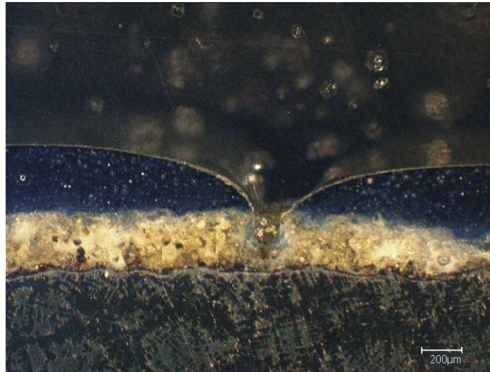
Figure 12 — Pinhole, cross section
