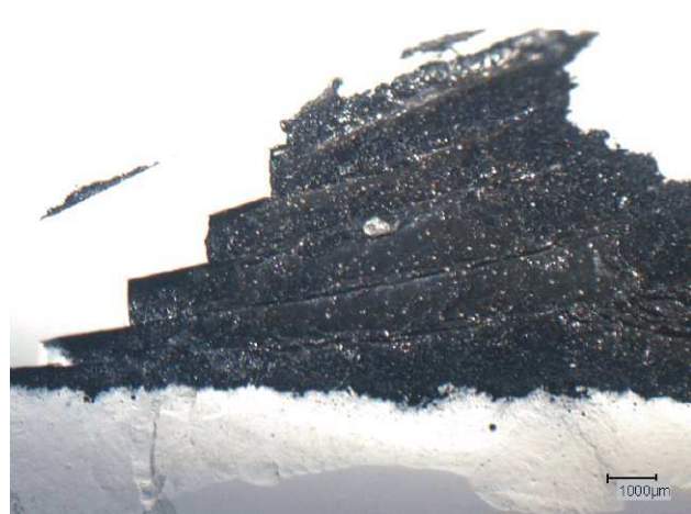
b) Chipping resulting from too high a compressive stress
