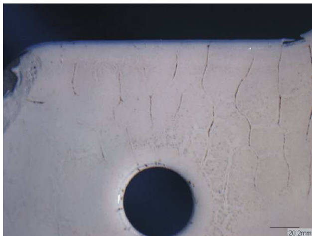
a) Cracks, top view
