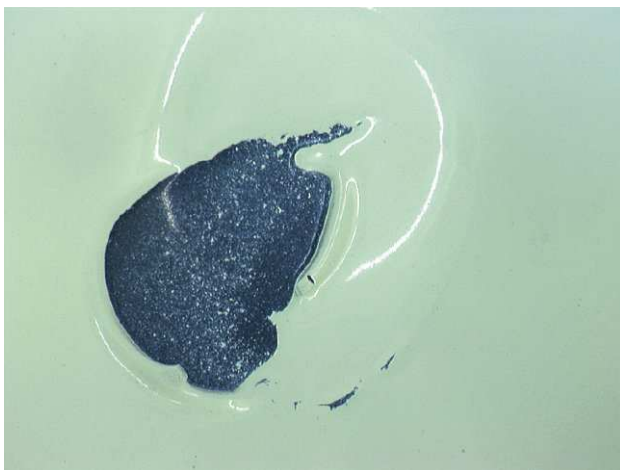
a) Crawling defect as a result of oil or grease
