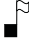
Figure 15 — Example symbol: point symbol composed of black square and flag symbolizing a school
