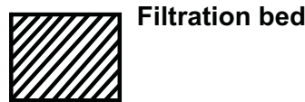
Figure 21 — Example symbol: complex area symbol with line symbol cross-hatching symbolizing a filtration bed
