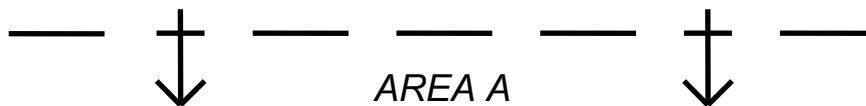
Figure 19 — Example symbol: complex line symbol with anchor point icons repeated along a line symbolizing a boundary to an anchorage area
