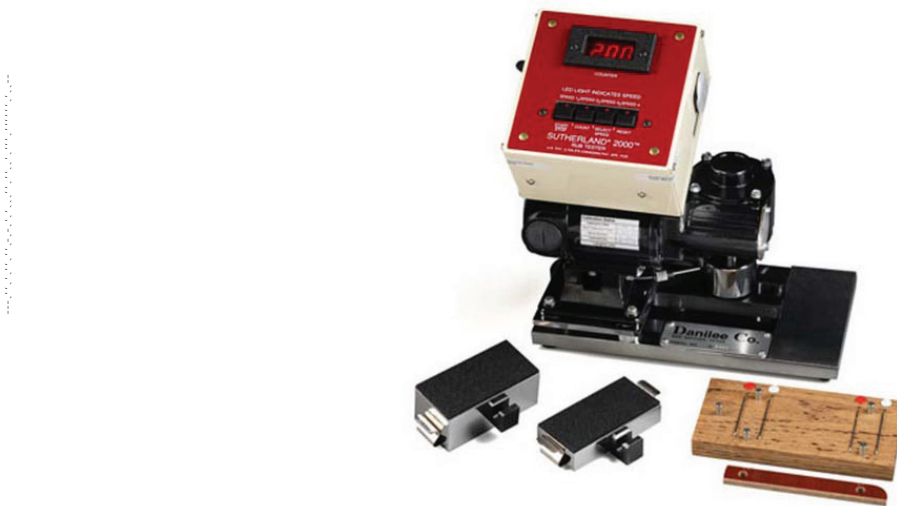
Figure A.1 — Test device described in ASTM D 5264, ASTM F 2497 and ASTM F 1571
