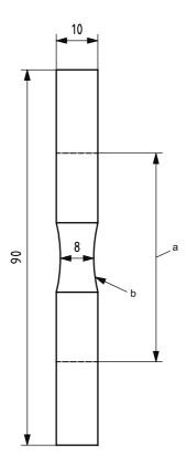
Figure 1 — New tensile specimen for the determination of tensile behaviour at high strains
