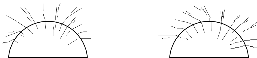
Figure B.6 — Fine hackle lines which may change direction at the crack front line
