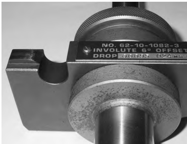
Figure 3 — 115 mm base circle diameter involute artifact
