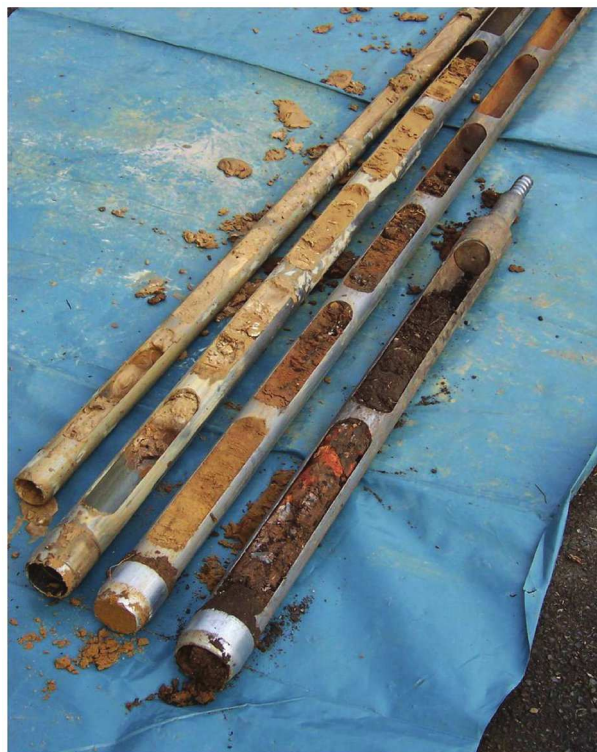
Figure C.13 — Window sampler tubes — Note reducing diameter with depth
