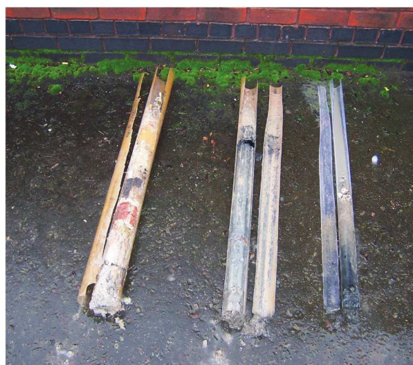
Figure C.14 — Plastic liners from windowless sampler cut open to reveal core
