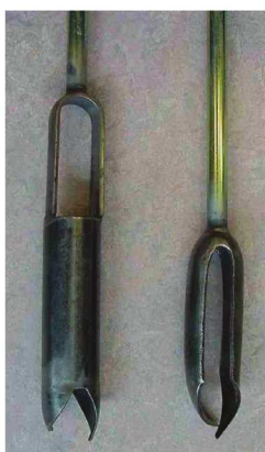
Figure C.3 — “Riverside” and gravel augers
