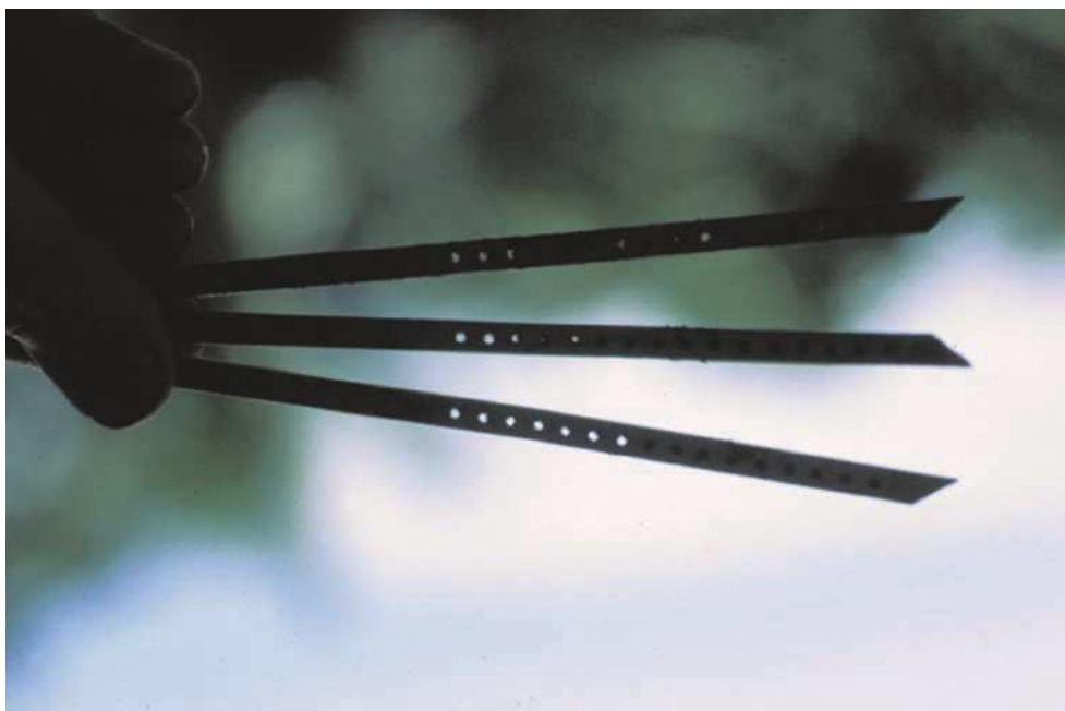
Figure 5 — Visual examination of an individual bait-lamina strip at the end of a test (Photograph: H. Hoefler)
