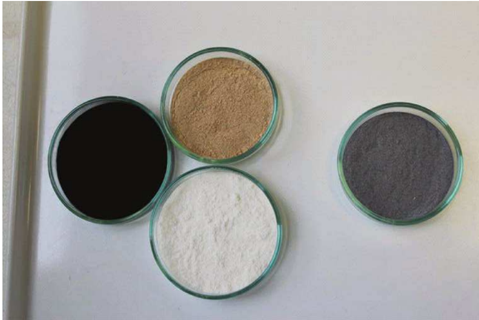
Figure 2 — Three individual materials (left: activated carbon; above: finely ground wheat bran; below: cellulose) and the mixture of the three components at right: the bait
