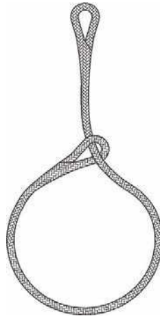
Figure 4 — Example of choker hitch
