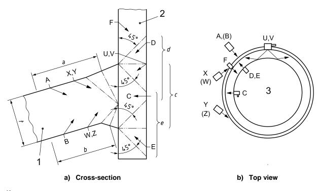
$\begin{tabular}{lll} \textbf{Key} \\ 1 & component 1, cylindrical shell/flat plate \\ 2 & component 2, nozzle \\ 3 & normal probe \\ A, B, C, D, E, F, U, V, W, X, Y, Z & probe positions \\ a, b, c, d, e & scanning zone width indicators \\ t & thickness \\ \end{tabular}$
