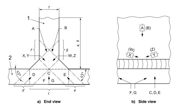
Figure A.2 — Structural T-joints
