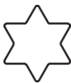
Figure 4 — Shapes of engaging part with implant bodies or connecting parts in torque transmitter: Hexalobular-shaped (star-shaped)
