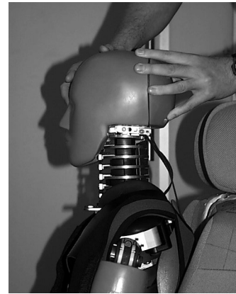
Figure B.12 — Head pushed backward until head is horizontal, nodding joint remains in extension
