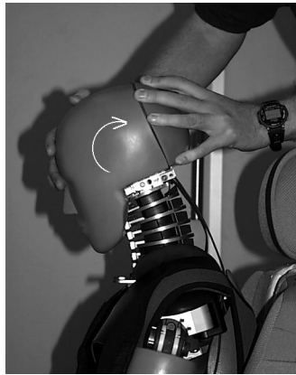
Figure B.11 — Head rotated backward until nodding joint extension stop
