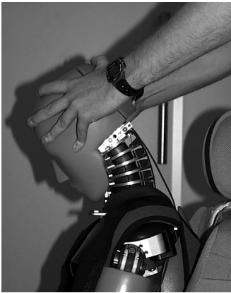
Figure B.10 — Head pushed forward, neck in maximum flexion
