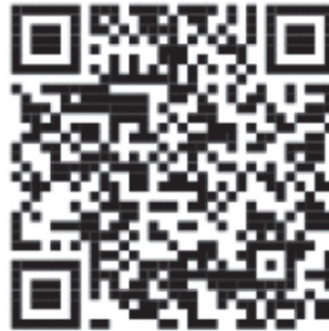
Figure B.5 — QR Code encoding the contents of MB01 and MB11 [ ]><RS>06<GS>25SUN043325711MH8031200000000001 <GS>1T110780<GS>Q21<GS>4LUS<RS><EOT>
