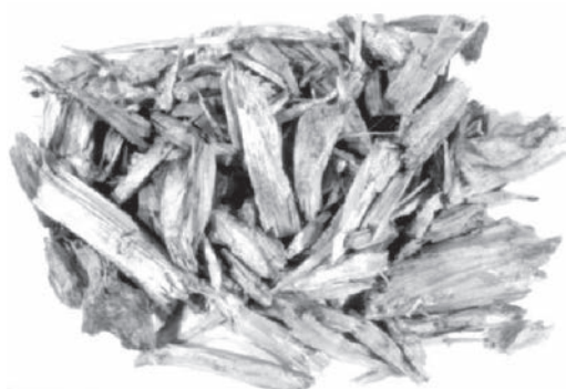
b) Hog fuel (crushed with blunt tools)
