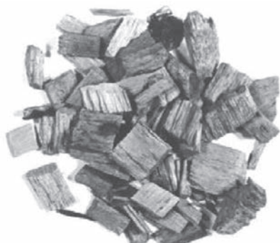
a) Wood chips (cut with sharp tools)
