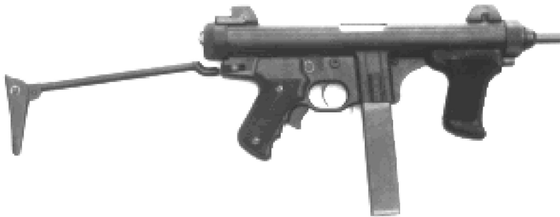
Figure A.14 — Submachine gun with blow-back action
