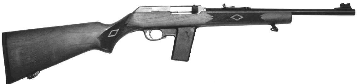
Figure A.12 — Semi-automatic rifle with blow-back action
