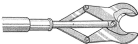
**3.1.4.2****spreading or jacking tool**
