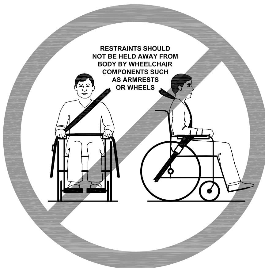
Figure E.2 — Example of warning label indicating improper positioning of occupant restraints
