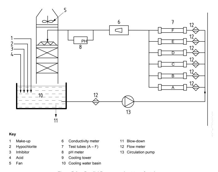
Figure B.2 — Parallel flow across heat-transfer tubes
