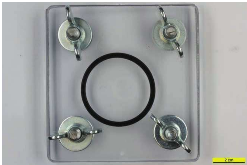
Figure C.2 — compression of O-ring using 4 screws
