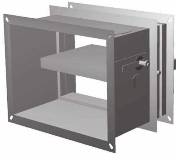
Figure 14 — Example — Air condition fire damper CSG-model made of CSG sheet metal primitives
