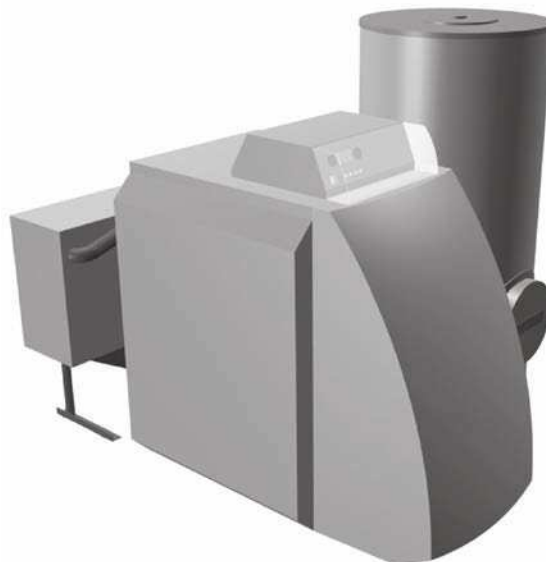
Figure 3 — Single product (heater with heat exchanger and water storage) as an assembly of components
