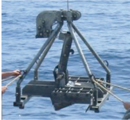
Figure A.2 — Example of a Hamon grab; image source: VLIZ (Flanders Marine Institute), reproduced with permission
