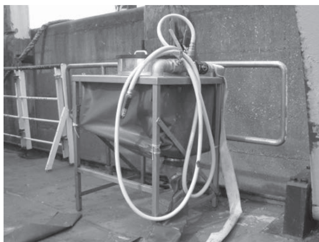
Figure A.7 — Example of a Wilson Autosiever; image source: VLIZ (Flanders Marine Institute), reproduced with permission
