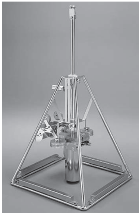
Figure A.6 — Example of a HAPS corer; image source: KC Denmark, reproduced with permission
