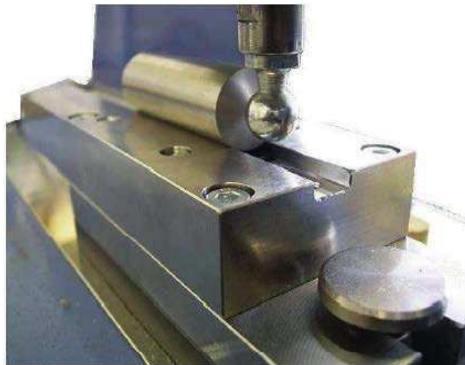
Figure C.2 — Mounted impact device with a cylindrical mass piece and pendulum bob
