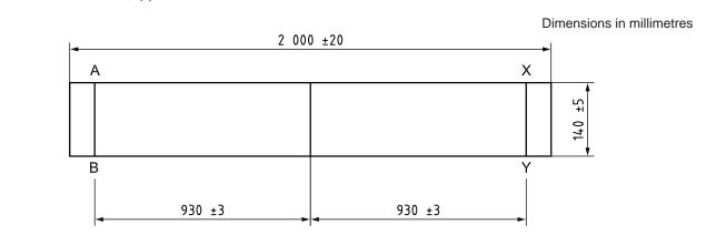
NOTE Line AB should be drawn on the opposite surface to line XY.
