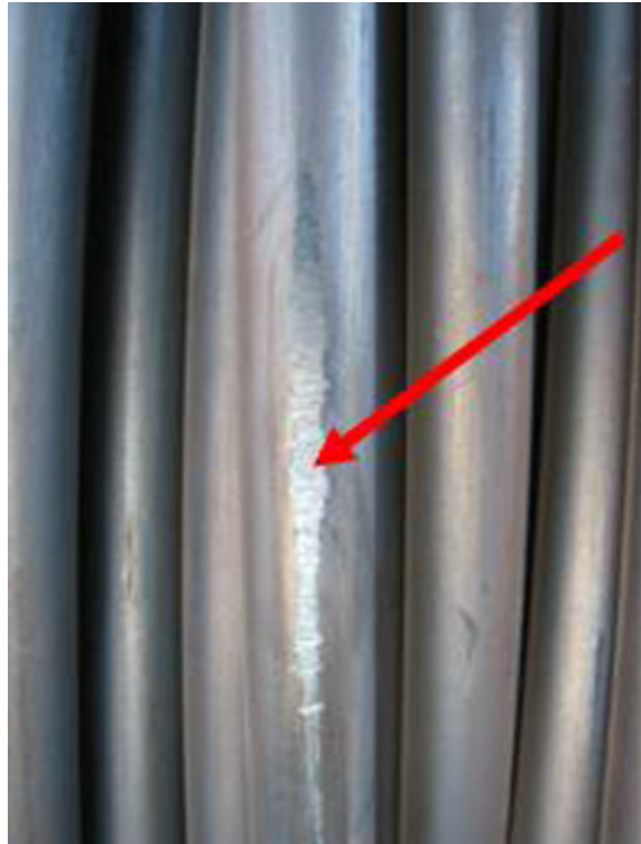
Figure C.1 — Abrasive damage caused by coil-to-coil contact
