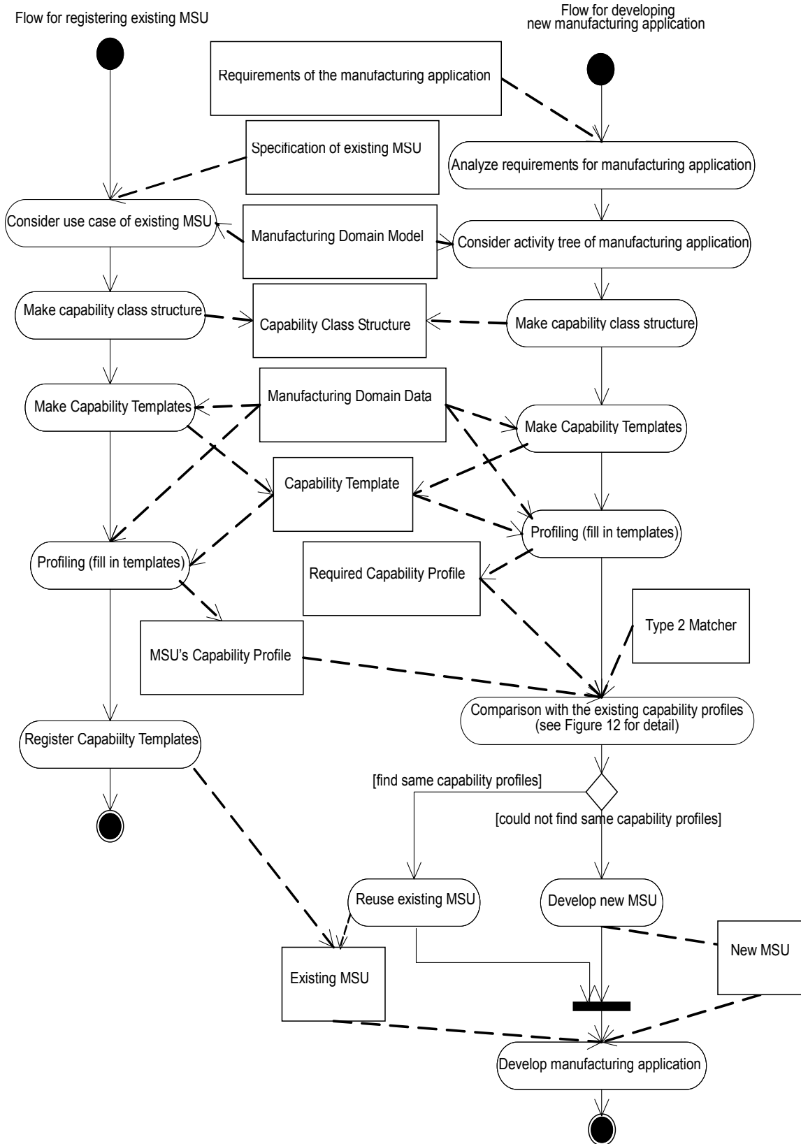
Figure 2 — Application development process with capability template, capability profile, and CCS
