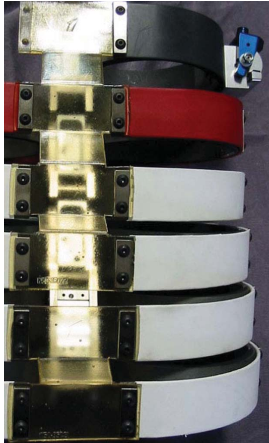
Figure A.25 — Shoulder rib is grey, the first thoracic rib is red, and the second and third thoracic ribs and abdominal ribs are white
