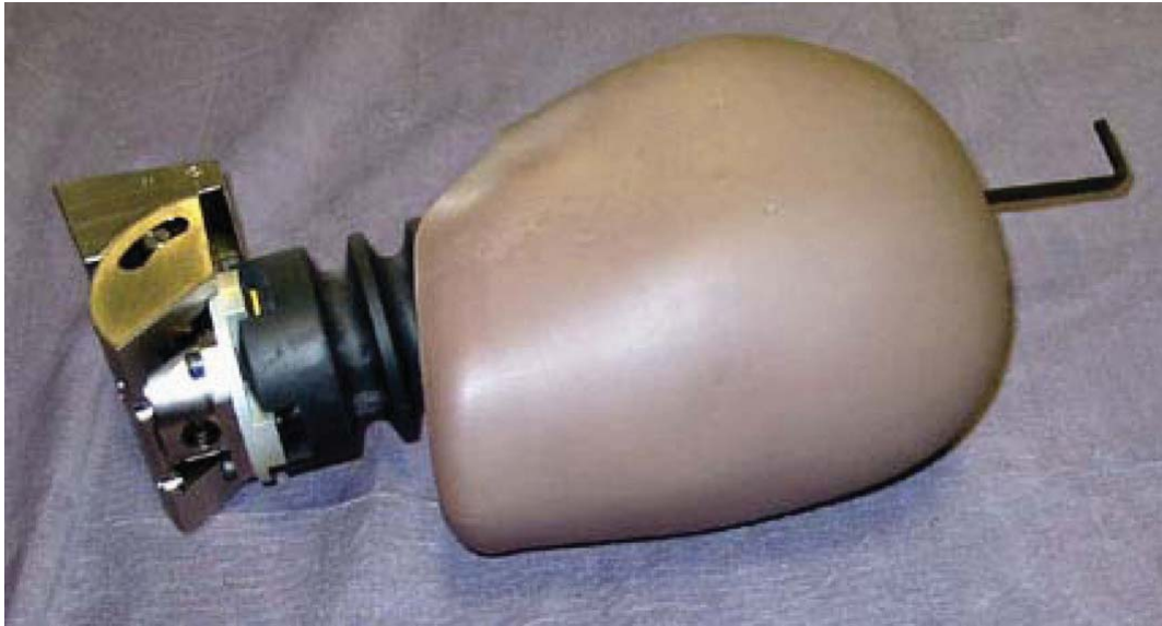
Figure A.2 — Removal of moulded head
