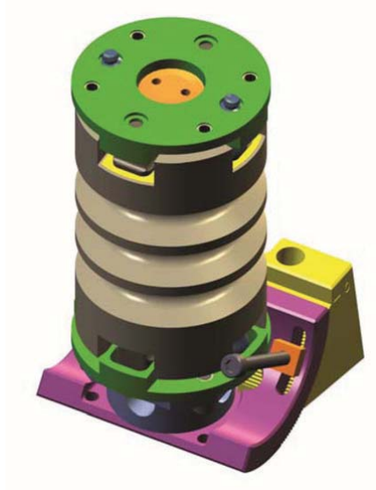
Figure A.8 — Removing lower neck bracket
