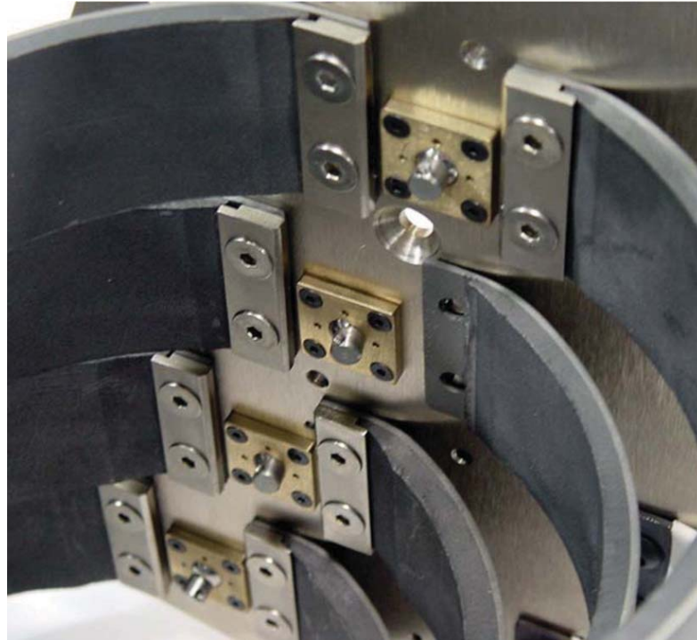
Figure A.24 — IR-TRACC ball joint assemblies are mounted to the struck-side plate of the spine box
