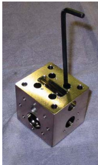
Figure A.69 — Separating the sacroiliac and lumbar spine load cell structural replacements
