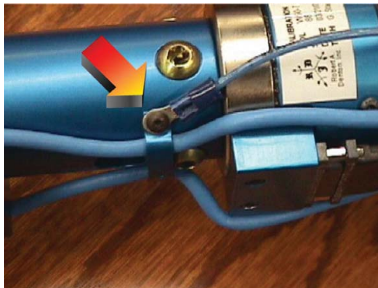
Figure I.9 — Tibia cable attachment
