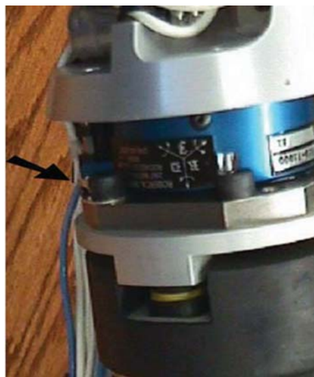
Figure I.1 — Cable attachment to the upper neck load cell
