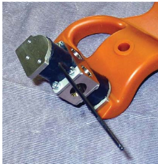
Figure A.61 — Separating pubic buffers from pubic load cell structural replacement
