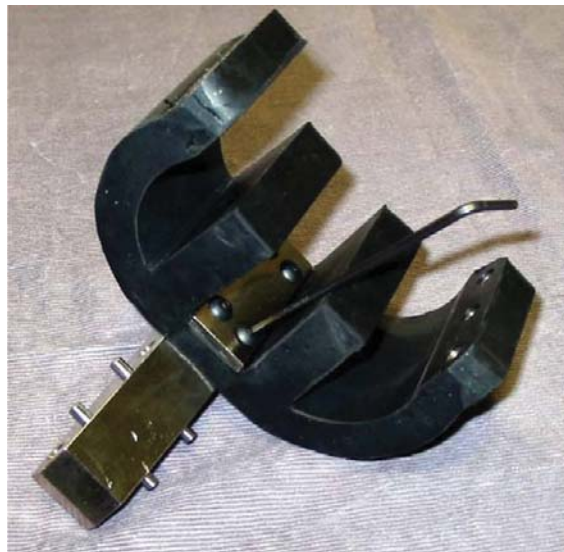
Figure A.63 — Separating the upper lumbar clamping plate and lumbar mounting wedge from the lumbar spine
