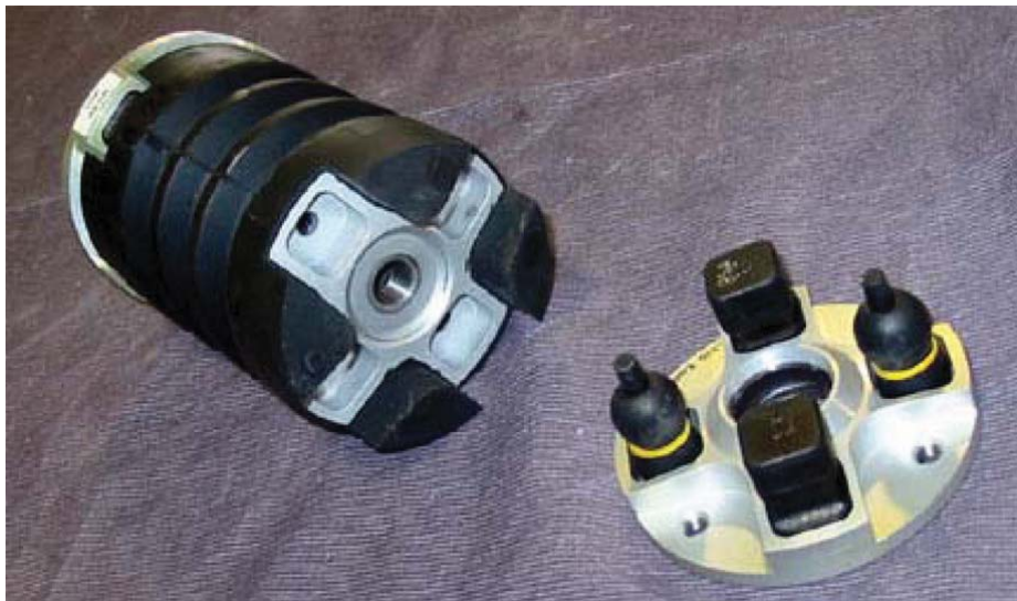
Figure A.11 — Neck dampers are free to be removed when interface plates are removed
