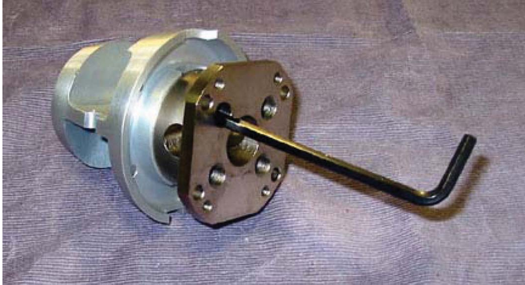
Figure A.4 — Removing upper neck load cell from instrumented head core
