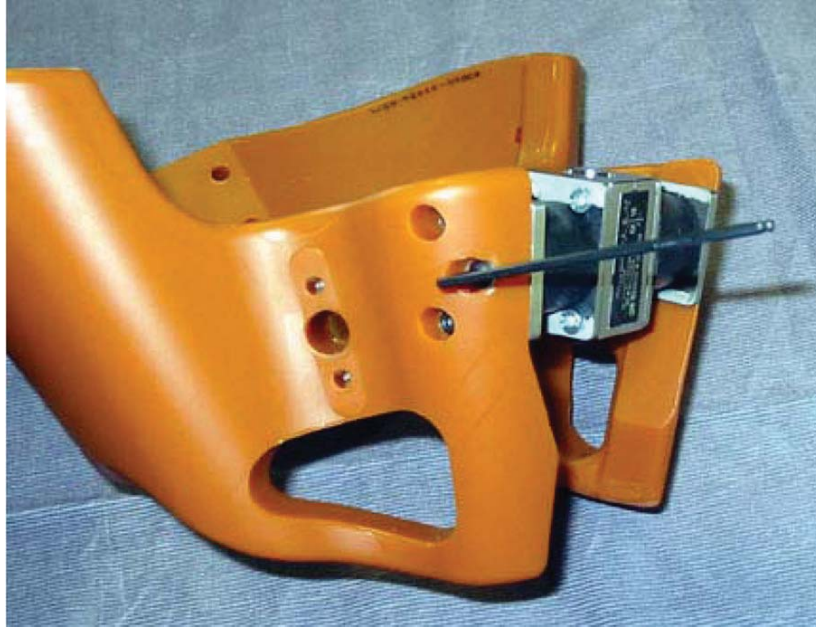
Figure A.60 — Separating moulded pelvis bone from pubis assembly
