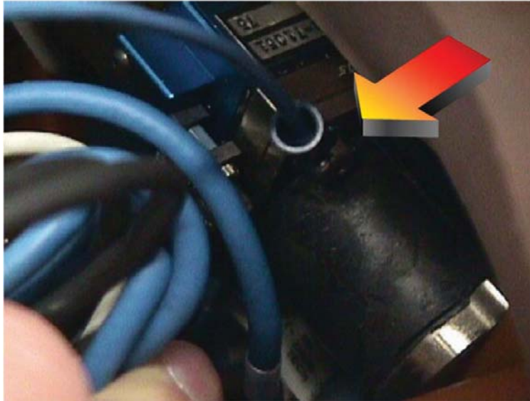
Figure I.6 — Pelvic load cell cable attachment
