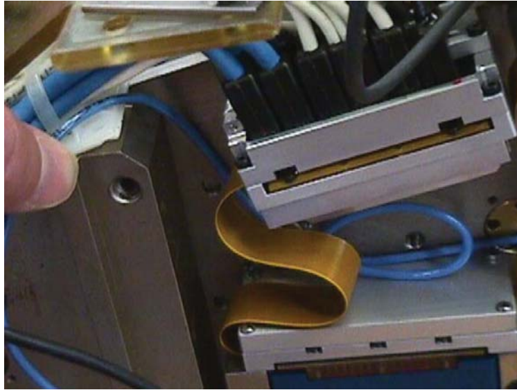
Figure I.2 — Spine box cable routing
