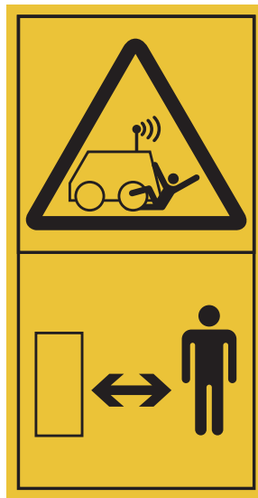
Figure A.1 — Example of machine safety label
