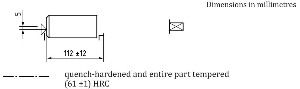
Figure 13 — Marking of a part which is locally heat-treated
