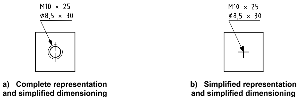
Figure 13 — Threaded hole with indication of cored hole diameter (hole bottom not specified)
