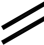
Figure 2 — Symbol for inclined joint
