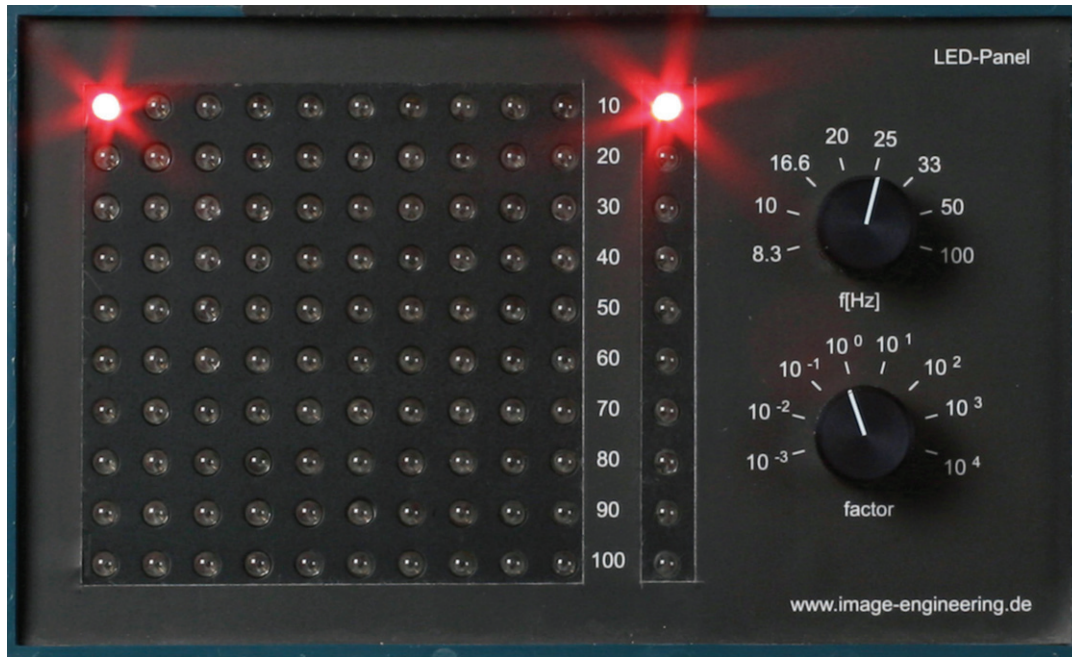
Figure B.3 — Sample device for a LED panel
