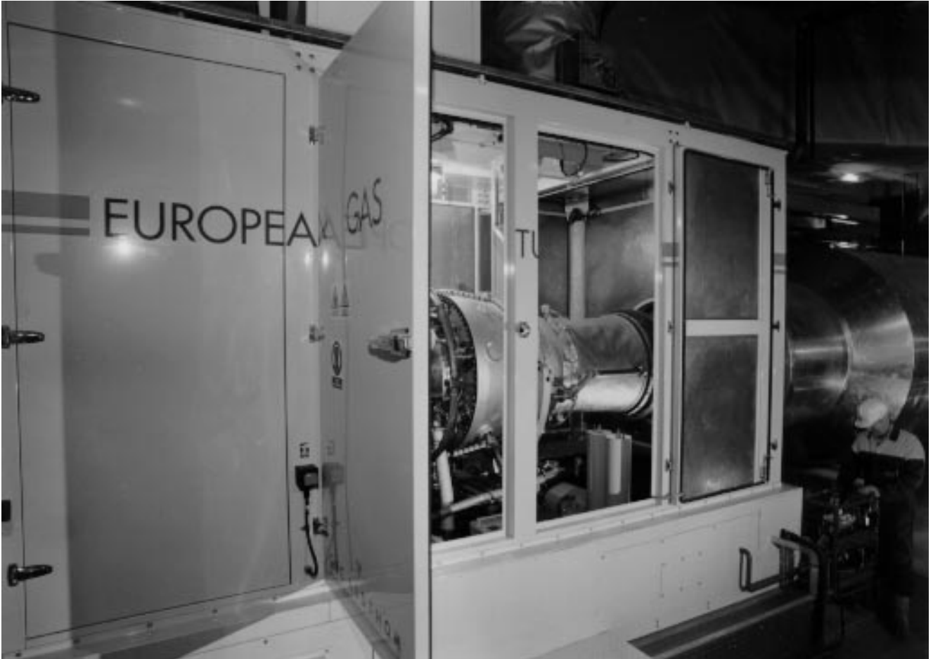
Figure B.11 — Gas turbine with enclosure, access panel open
