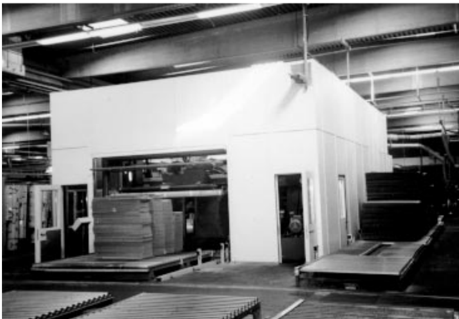
Figure B.10 — Production line for corrugated cardboard without (top) and with (bottom) enclosure
