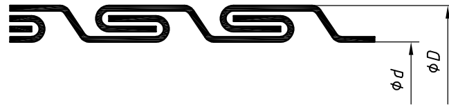
Figure 3 — Cross-Section of a type DOU, double overlap, unpacked hose
