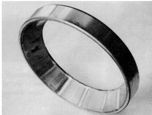
Figure 22 — Plastic deformation on a tapered roller bearing raceway produced by overloading
