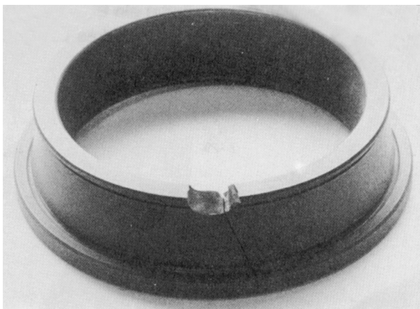
Figure 27 — Forced fracture caused by a direct hammer blow
