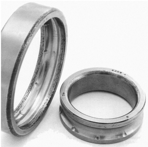
Figure 23 — Overloading during mounting
