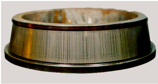
Figure 19 — Craters formed by current leakage resulting in fluting
