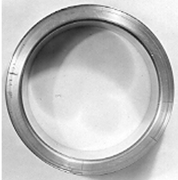
Figure 32 — Thermal cracking on an inner ring face
